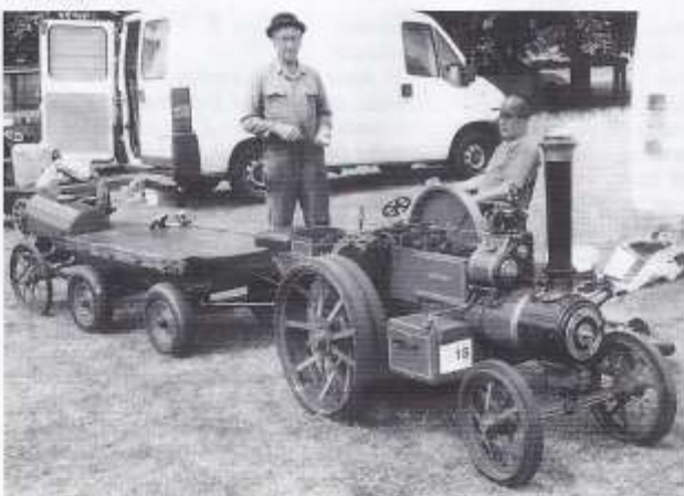
Chris Smith's 4" scale Burrell Single Crank Compound Road Locomotive and 4" scale Fowler Water Cart. The engine was built between 1996 and 2000.
