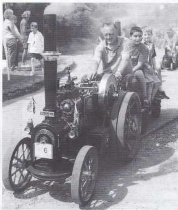
Pictured is George Toyne's 4" scale Foster DCC Road Locomotive.
