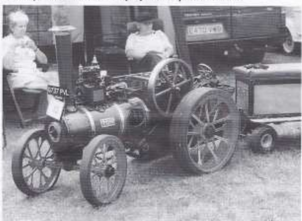
T. Landsbury's 4" scale Garrett 7NHP Agricultural Engine, built over 2 years as a retirement project, completed in 1998.
